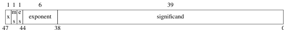
Figure 570.2: The Unisys A Series [5] uses the same representation for integer and floating-point types. For integer values bit 47 is unused, bit 46 represents the sign of the significand, bits 45 through 39 are zero, and bits 38 through 0 denote the value (a sign and magnitude representation). For floating values bit 47 represents the sign of the exponent and bits 46 through 39 represent the exponent (the representation for double-precision uses an additional word with bits 47 through 39 representing higher order-bits of the exponent and bits 38 through 0 representing the fractional portion of the significand).
